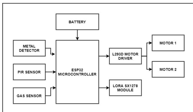
Fig -1: Block Diagram of Robot
