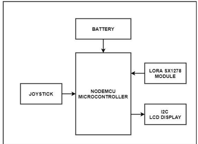
Fig -2: Block Diagram of Remote-control
