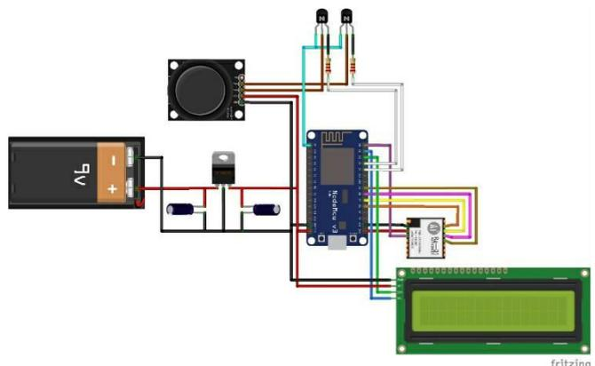
**Fig -3:** Descriptive Diagram of Remote Control
